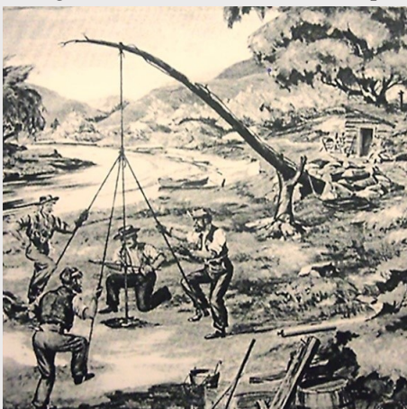
Rudimentary spring pole system. From F. Gerali (2019). Spring Poles , Engineering and Technology History Wiki. [Online] Available: https://ethw.org/Spring_Poles .
